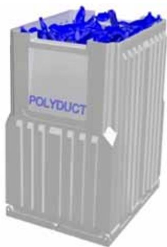
Fig. 4. 1,5m 3 container saturated by PET bottles compressed by leg
