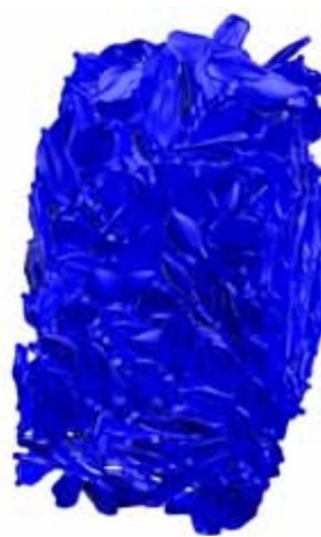
Fig. 5. Form of PET bottles compressed by leg in 1,5m 3 container
