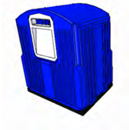
Fig. 2. 3D design of 1,5 m 3 selective waste gathering container
