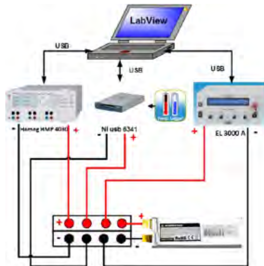
Fig. 5: Scheme of battery testing equipment
